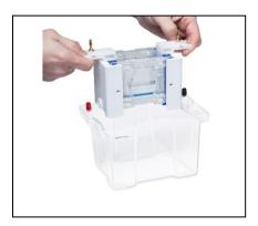
NOTE: It is best to turn the cams in opposite directions to each other. Do not overturn as this will cause the glass plates to push upwards and the assembly will be more likely to leak. The unit is now ready for gel preparation and pouring.
